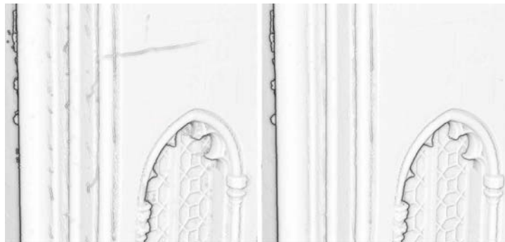
Figure 4. SOR filter. In the left figure we observe isolated points in the cloud "floating" by the space, that when applying the filter disappear as it is seen in the right figure.
