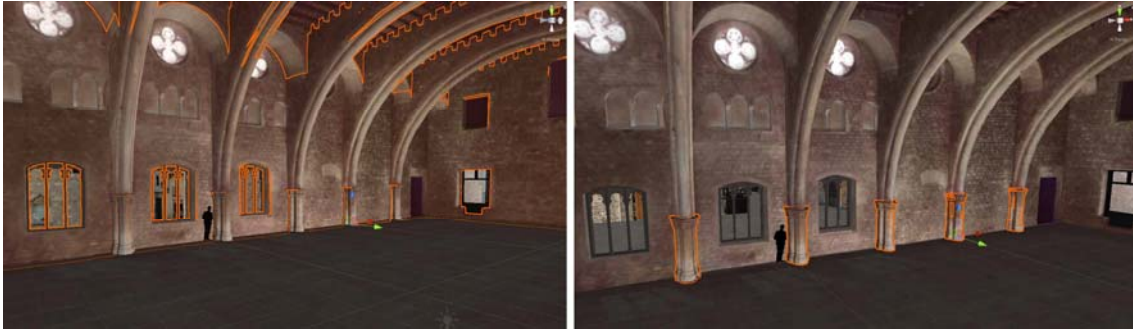
Figure 7. Architecture model. The model from the mesh, where repeating elements can be moved, aligned or edited as separate objects.
