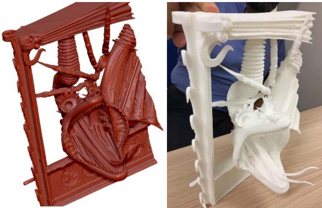
Figure 11: Left: 3D printing grid (1.5 million polygons). Right: picture of the printed model
